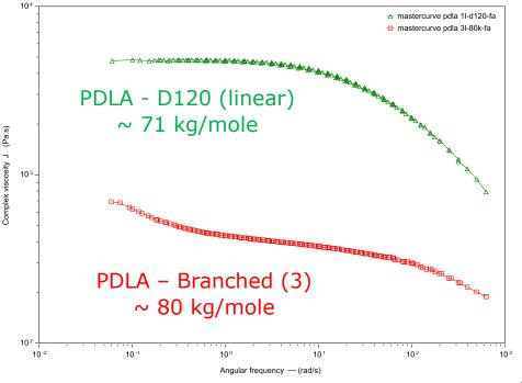
Complex viscosity of branched polymer is lower than of linear polymer.
