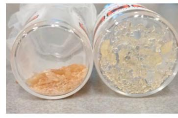
Polyhydroxyurethane with Tg-value above room temperature (left) and around room temperature (right)
