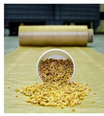
Testbatch foil and granules based on chitin
